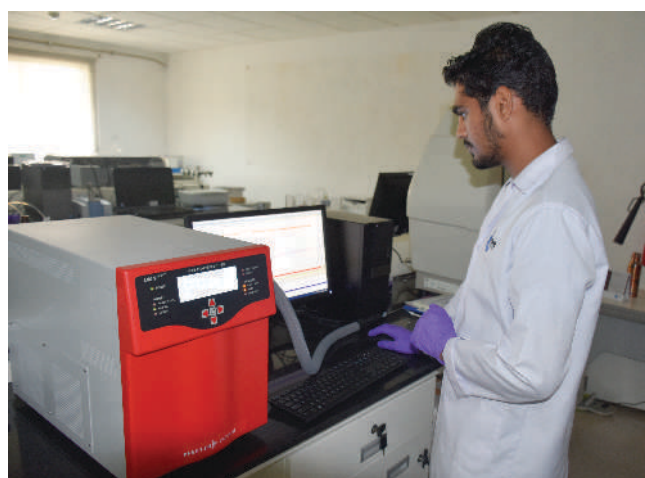
▲ Gas Chromatography Mass Spectrometer (GC-MS), OmniStar™ GSD 320 O1, 1–100 amu
