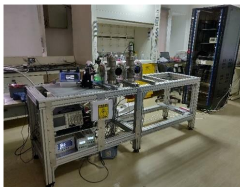
Cryogenic ion trap setup under construction
